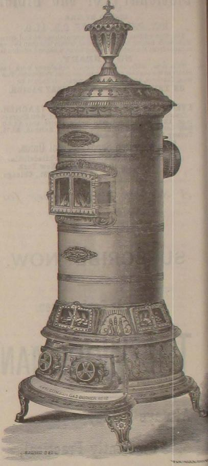
All similar stoves have been constructed with the old rotating grate, and to get clear of clinkers each week the fire had to be dumped, but with our Anti-Clinker Grate we present a cheap stove by which clinkers can be removed without dumping, and a perpetual fire kept going, while the base of the stove is always hot. These Stoves have clay cylinders; retain the fire at a lower temperature and consume less coal than an iron-lined cylinder.
